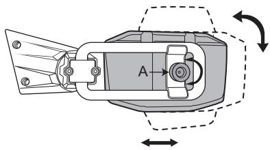
01: Adjust the screw A to change the direction or position of the mirror.
