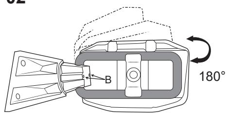
02: Adjust the screw B, you can swing frame front and back by 180°.
