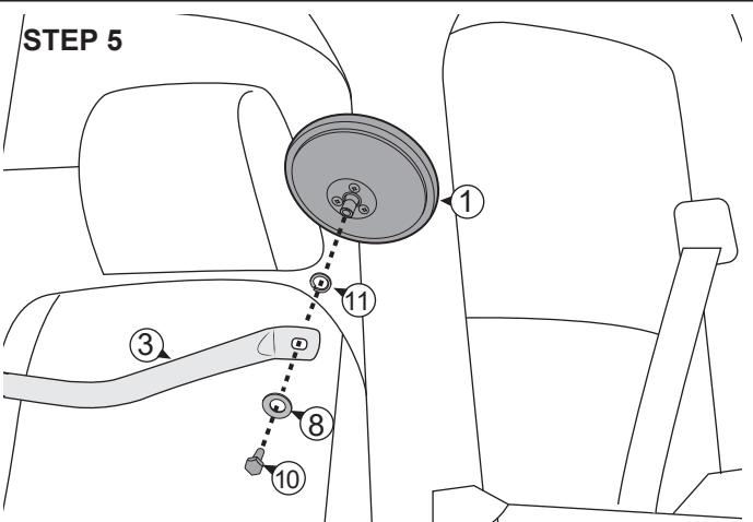
Attach mirror ① to flat side of arm ③ using the bolt ⑩, flat washer ⑧ and lock washer ⑪.
