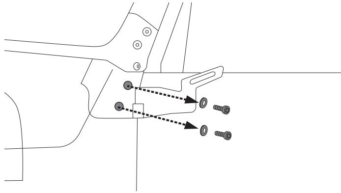
Remove two original flush mount torx head bolts and washers just in front of door hinge.
