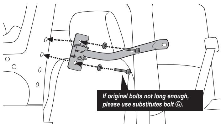
Use the two original bolts and washers just removed to fix the bracket on the flat side.
