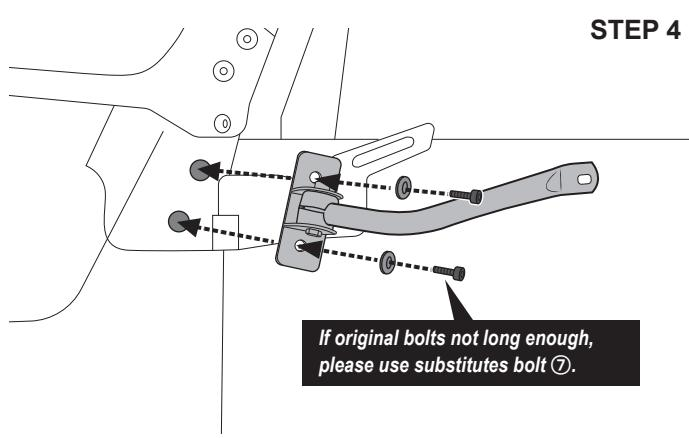
Use the two original bolts and washers just removed to fix the bracket on the flat side.
