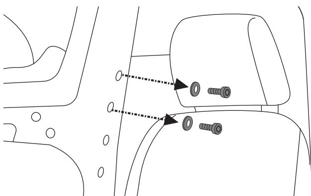
Remove two original flush mount torx head bolts and washers just in front of door hinge.
