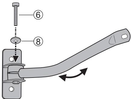
Install the bolt ⑥ and flat washer⑧, tighten the bolt, don't over tighten them, you can adjust them as needed.
