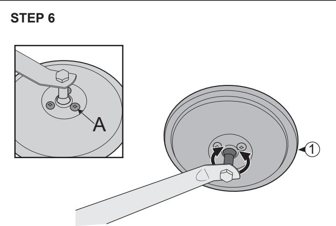
Adjust the mirror ① head into desired position, tighten three screws [A], DO NOT over tighten. The mirror ① should be tight but able to be adjusted if needed.
