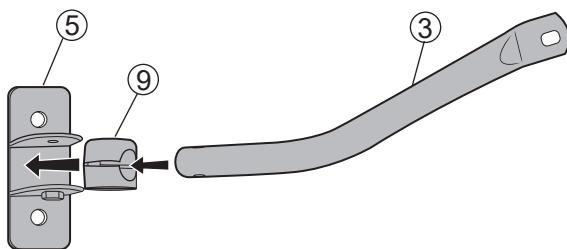
Assemble the right mirror arm③, billet bushing⑨ and mounting bracket⑤.
