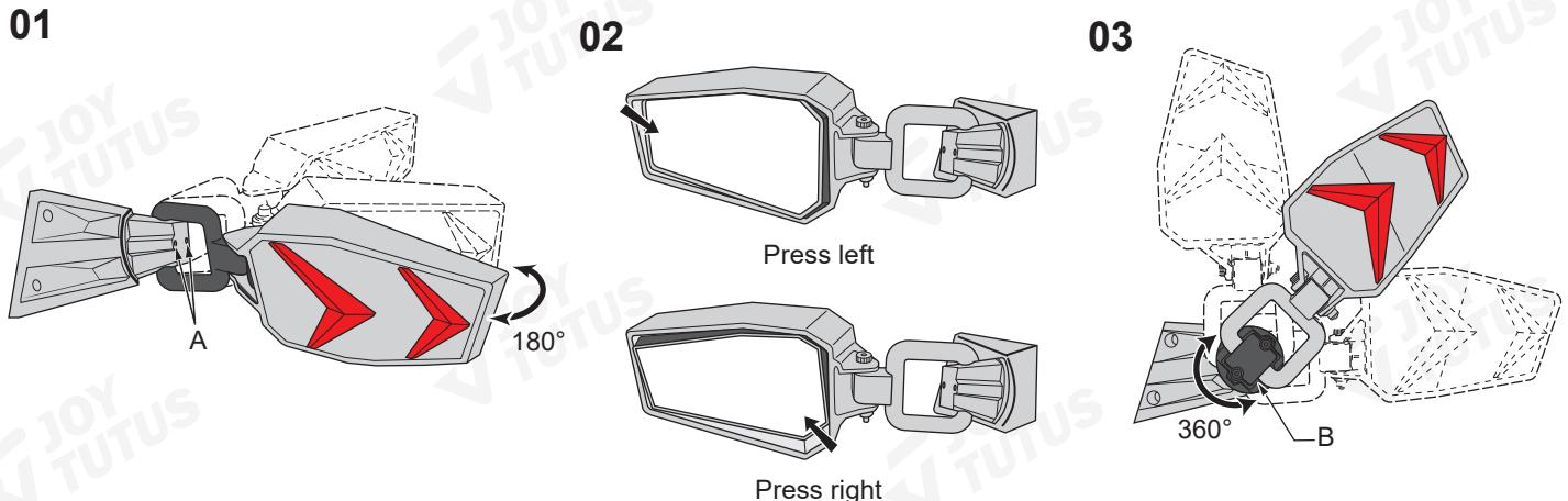
**01)** Adjust the screw A, you can swing frame front and back by 180°.
