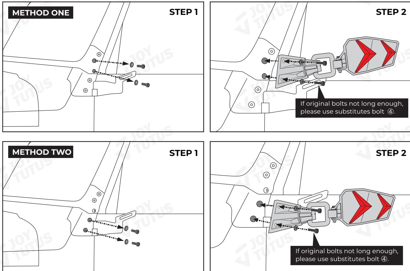
**STEP 1:** Remove two original flush mount torx head bolts and washers just in front of door hinge.
