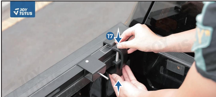
4. Lock the mounting clamp on the corresponding dashed line mark.
