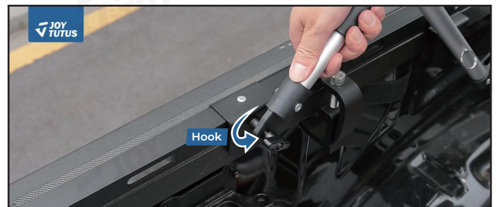
5. Installation of brackets (Driver and passenger side)
