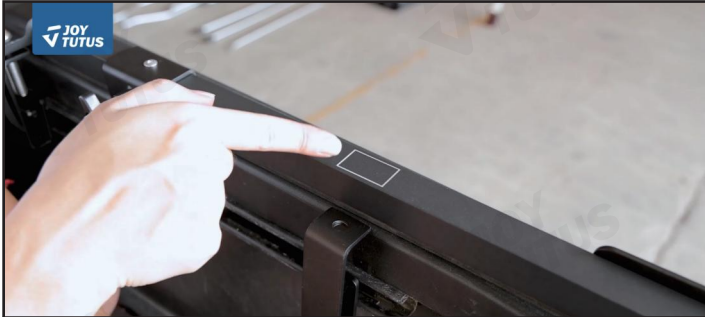
4. Lock the mounting clamp on the corresponding dashed line mark. (NOTE: Do not change the position of the mounting clamp arbitrarily. It may cause interference with the support structure.)
