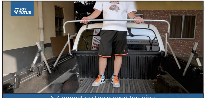
6. Connecting the curved top pipe Insert the top bending rod ⑨⑩ into the connecting bracket ⑤⑥
