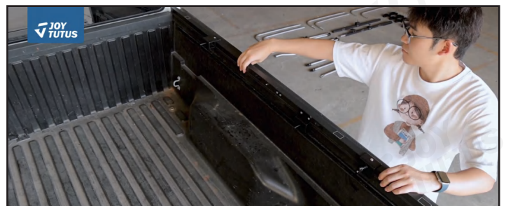
3. Place the base on the truck bed, with both ends corresponding to the respective positions on the truck (left and right bases should be symmetrical).
