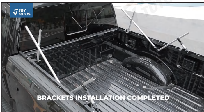
5. Installation of brackets (Driver and passenger side)
