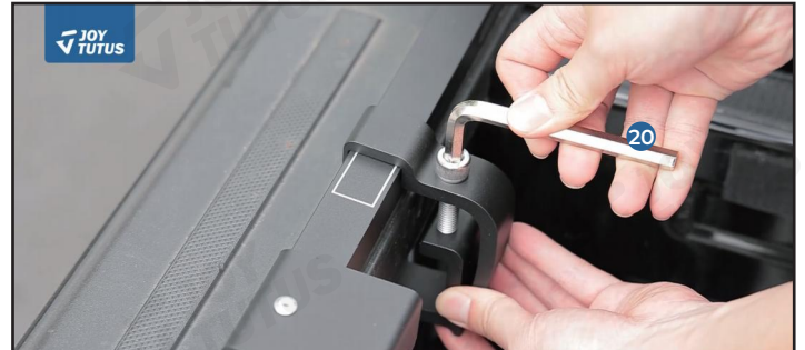
4. Lock the mounting clamp on the corresponding dashed line mark.
