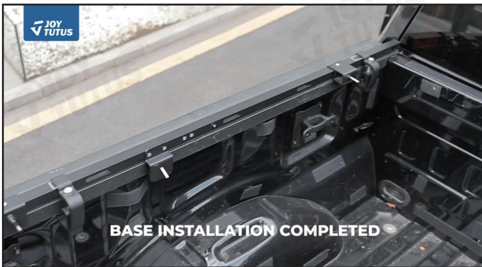
4. Lock the mounting clamp on the corresponding dashed line mark.
