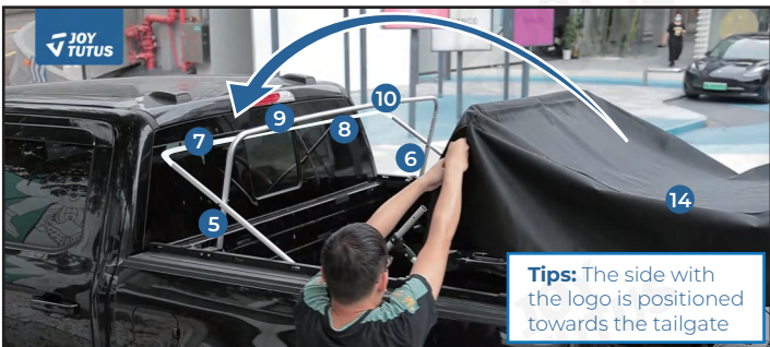
9. Wrap the cover around the bracket
